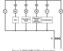
Figure 2: RAK147P1 6-Wire Connection
